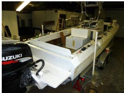
I built a very useful leaning post-live well-ice box-fresh water holding tank-trash bin out of plywood, epoxy and Lexan viewing window, where just a hard leaning post was mounted before. Added jump seats to the back, where wet tail was previously. Now there's room for four guests to sit or someone could lie down at the back end. Plus there's about three extra feet now on back to fish or relax.
