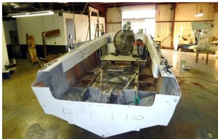
Then I started building new flooring using Baltec Airex panels & epoxy sandwich construction methods. Moved the console forward by 30" to get better balance. Cut out the fish box and applied two layers of insulating foam to its backside. While the floor was out, filled the hollow lifting strakes with crack sealing epoxy, and bolstered all the
