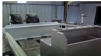
Final fairing and smoothing has begun, along with detail work for the seams around the new leaning post, the new in-floor storage holds, and painting using a two-part automotive urethane plus clear-coat from a HVLP gun. Anticipated completion of these upgrades is another month or so – final item will be renaming the boat to "Deep Eddy" I feel the boat will provide me many additional years of enjoyment and adventure.
