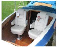
When the seats arrived, they were test-fitted in place. The pedestals are through bolted in the floor. An access hole was cut directly behind the pedestal mount in order to install the backing plates and have access to the nuts. The holes were filled with sealed deck plates to keep any water out. It was quickly discovered that the floor (formerly the v-berth base) was not flat. The starboard pedestal leaned about 2° towards
